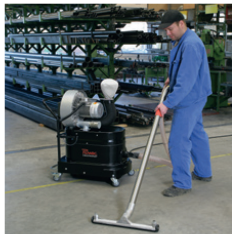
R01 S 015 explosive dust in warehouse cleaning
