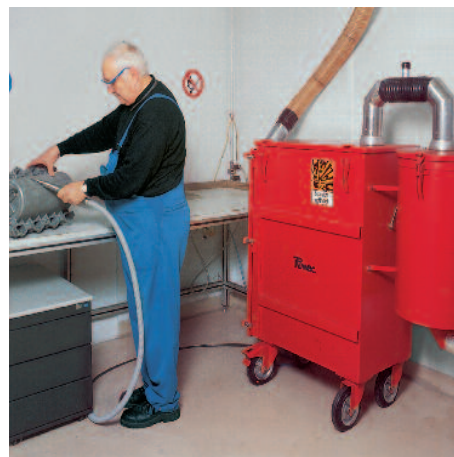
NA 250 sheet steel with residual dust filter in automotive supply/production
