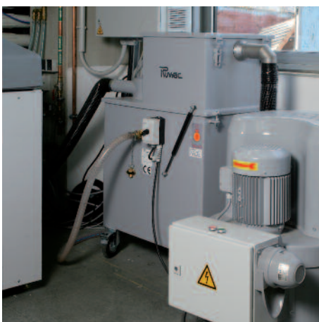
NA 250 sheet steel without residual dust filter, with vacuum unit in plastics processing
